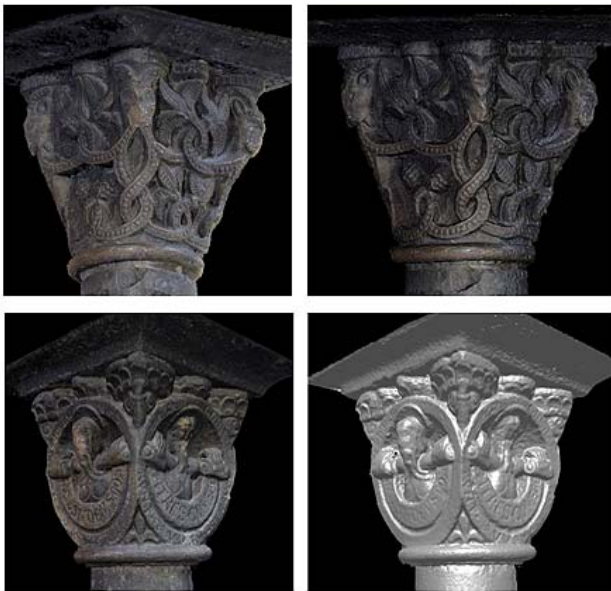
Figure 10. Different types of 3D model visualization: RGB point cloud (top and bottom left); photo-realistic (top right) and grey shaded models (bottom right)
