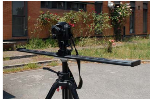
Figure 5. ZScan System used for data acquisition, with 0,90 m calibrated bar for camera sliding
